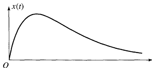
Figure 5.12 Overdamped motion in which the oscillator is kicked from the origin at t = 0 . It moves out to a maximum displacement and then moves back toward O asymptotically as t \rightarrow \infty .
